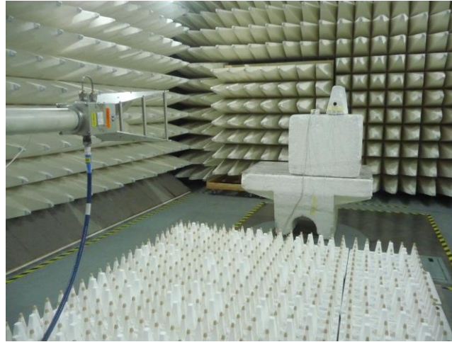
Photograph No.3 Setup for carrier field strength, spurious emission field strength measurements in the anechoic chamber above 1000 MHz
