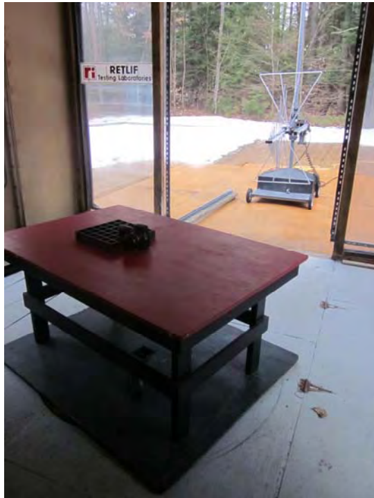
Vertical Antenna Polarization, 1 to 4 GHz
