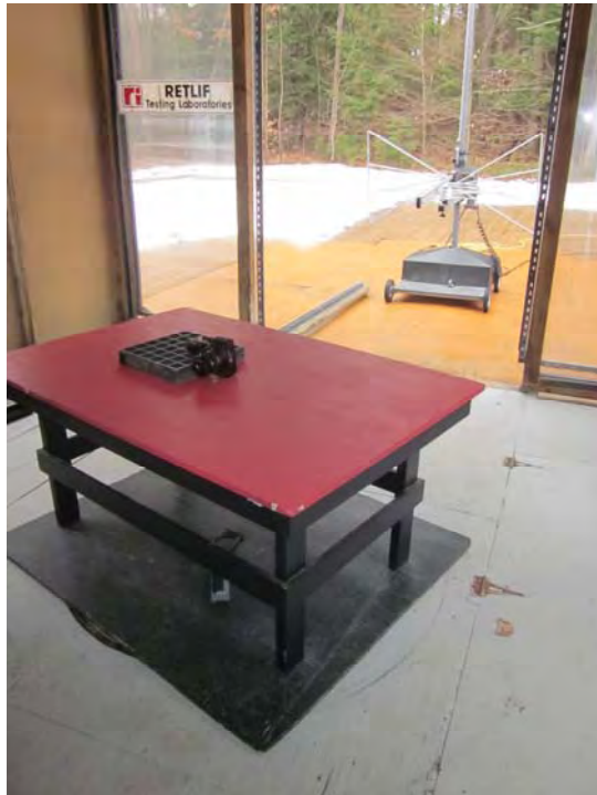
Horizontal Antenna Polarization, 30 to 1000 MHz
