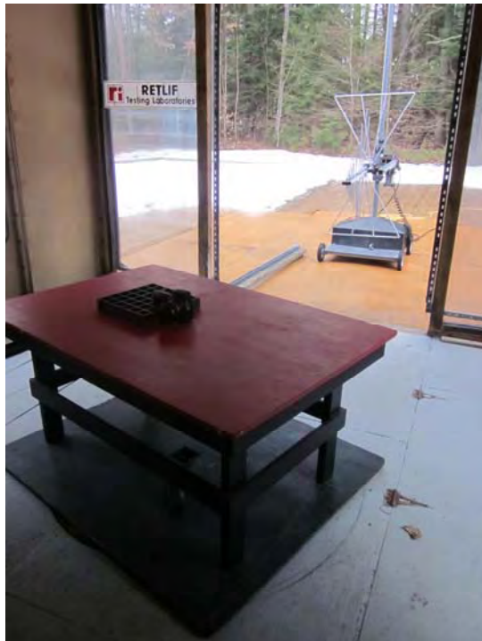
Vertical Antenna Polarization, 30 to 1000 MHz
