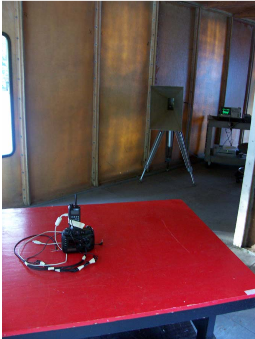
Radiated Emissions Setup Photograph
