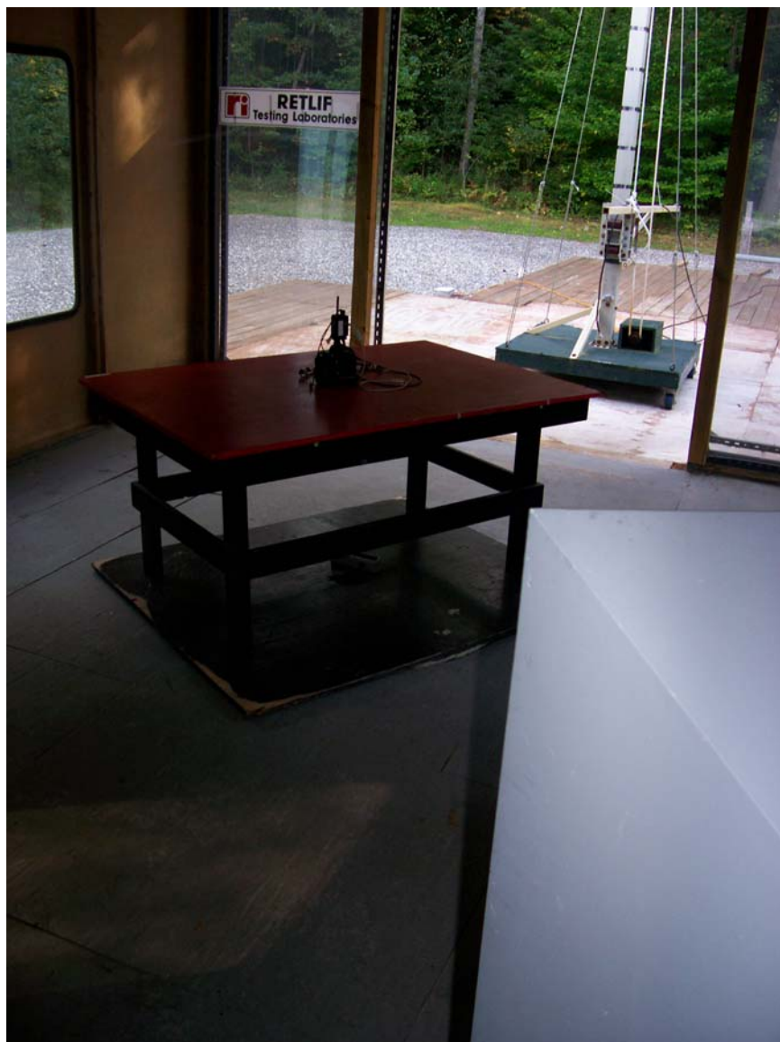
Radiated Emissions Setup Photograph
