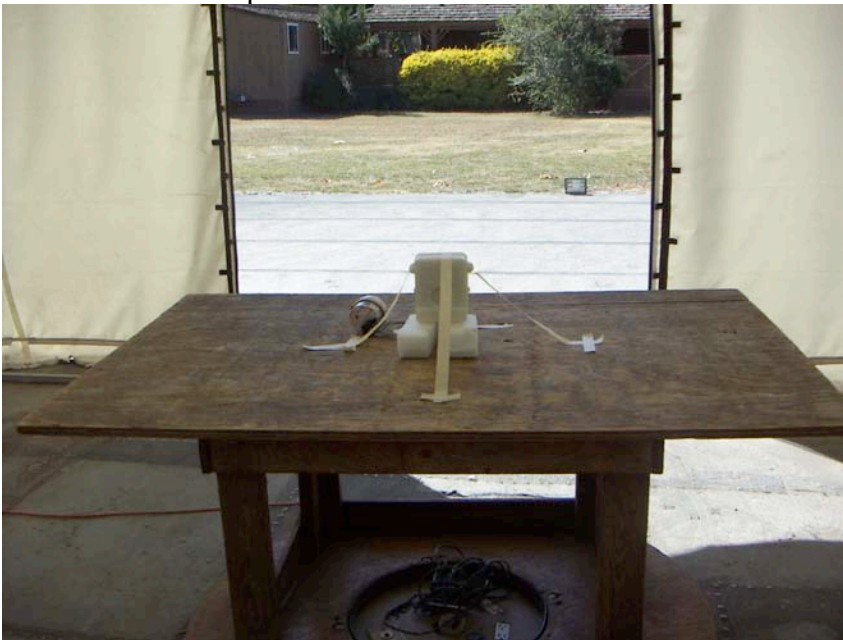
Radiated emissions, open area test site Above 1 GHz except for TX 3 rd harmonic emissions
