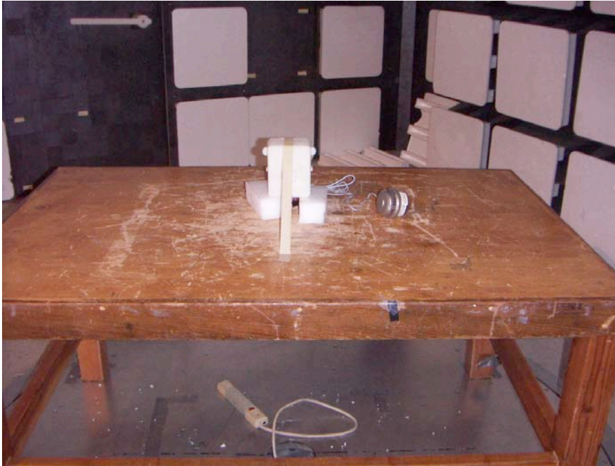
Radiated Emissions, anechoic chamber Below 1 GHz and 3 rd harmonic TX emissions
