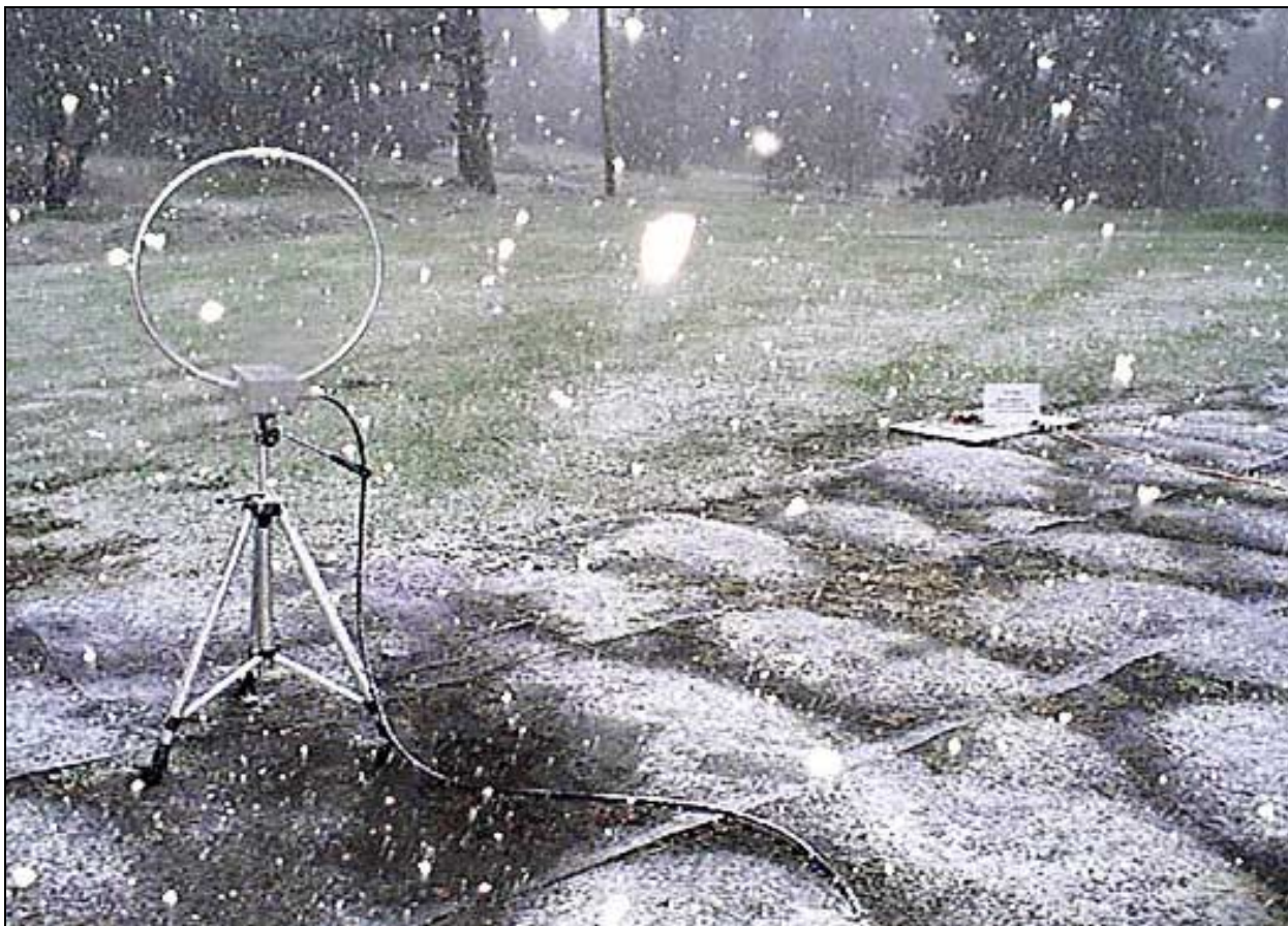
Radiated Emissions - Front View with Magnetic Loop Antenna
