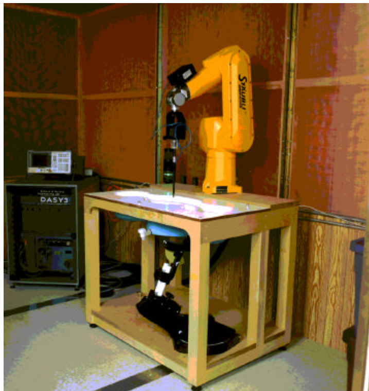
Figure 4. DASY3 SAR Measurement System
