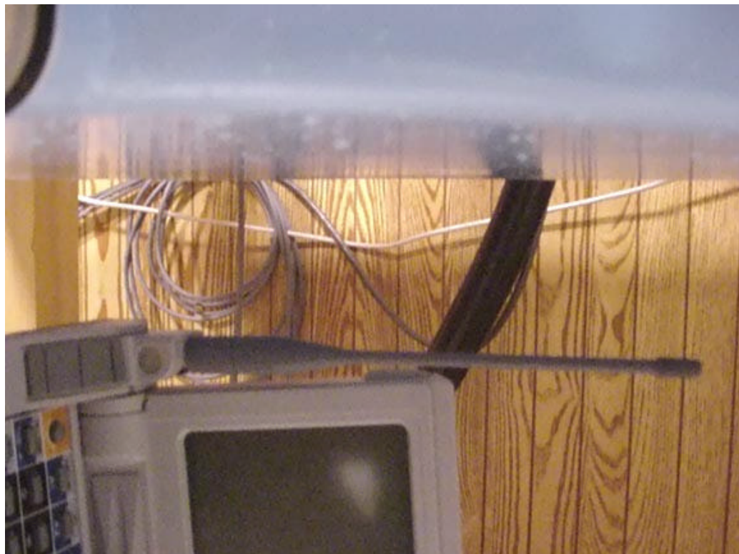
Fig. 6. SAR test setup with 5cm spacing between the antenna and planar phantom surface.
