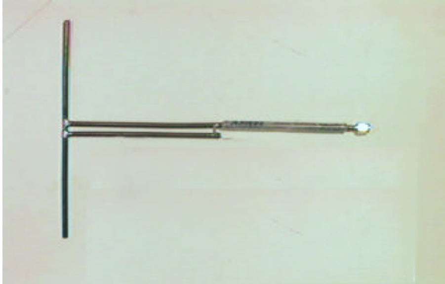
Reference Dipole Antenna Used for ERP Measurement
