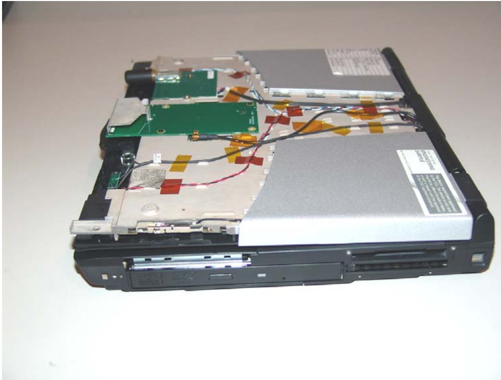
IX600 Close Up of Main WLAN antenna above
