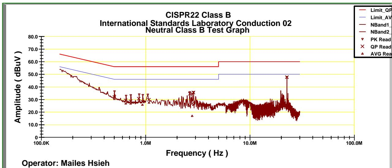
\* NOTE: During the test, the EMI receiver was set to Max. Hold then switch the EUT between Main antenna , Aux antenna Channel 1 , 4, 5, 8 ,9,12 of Normal Mode and Channel 1, 2, 3,4,5 of Turbo Mode to get the maximum reading of all these channels.
