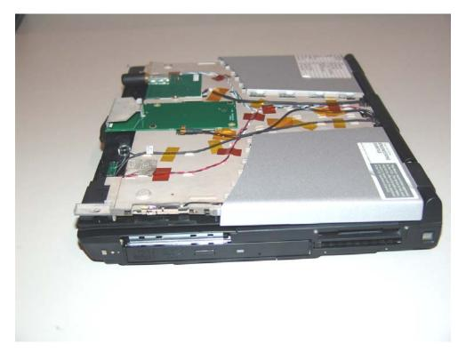
IX600 touch pad/keyboard cover flipped up, WAN radio located lower right side, WAN edge connector of module only partially visible
