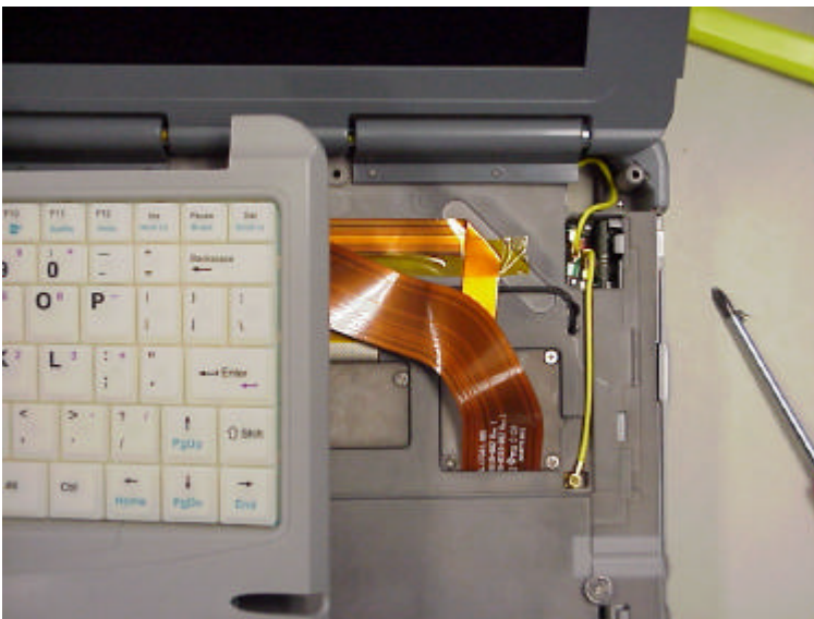
Outside the magnesium case and under the keyboard bezel a 3.8 inch cable routes to the cradle contact board that uses the same mechanical switch as the IX250. From the cable a 17.5 inch cable routes up through the display hinge.
