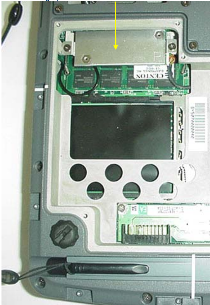
Photograph A.1-5 - Internal Bluetooth Location
