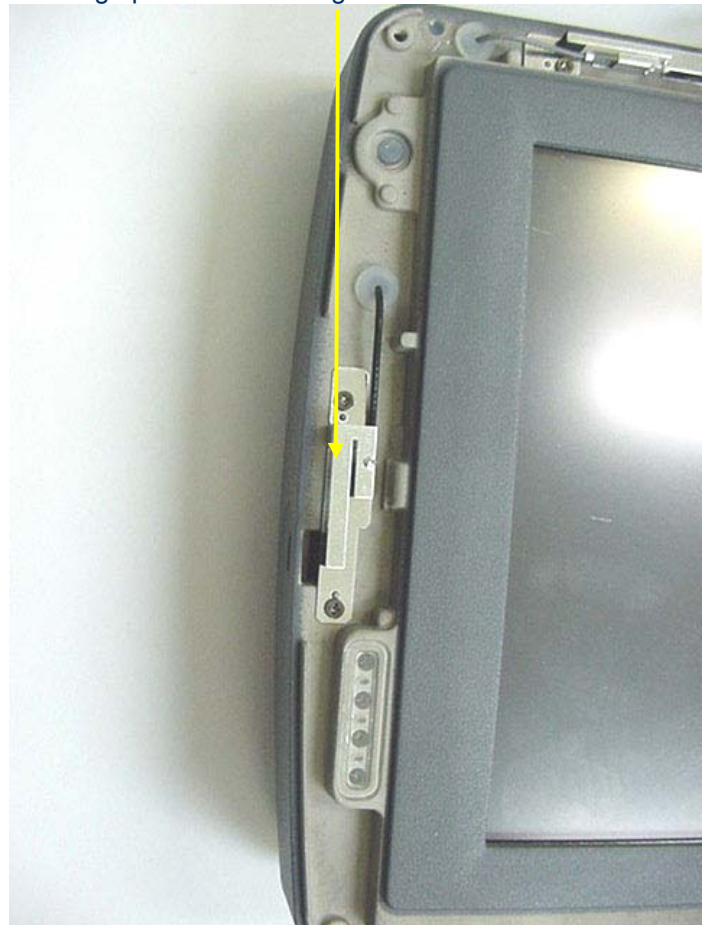
Photograph A.1-6 - Left Edge Bluetooth Antenna Location
