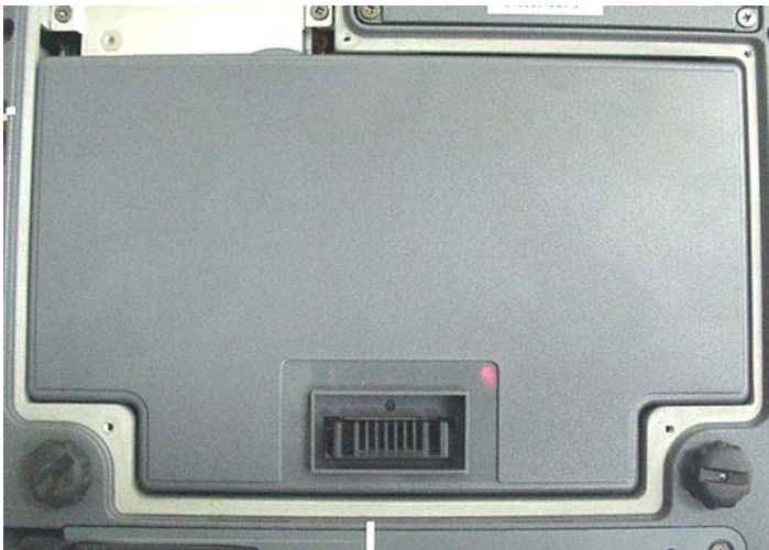
Internal Li-ion Battery 11.1 V, 3600 mAh (Model: T8M-E)
