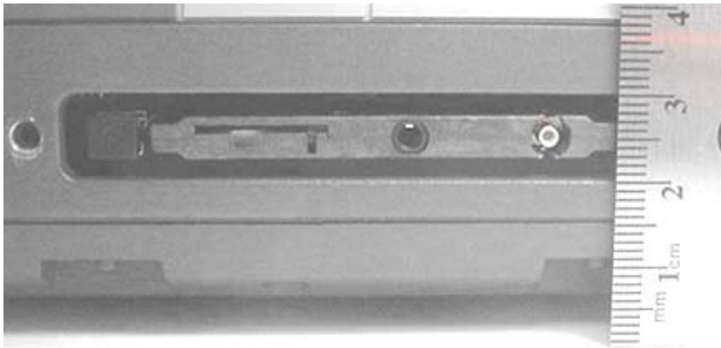
PCMCIA Slot-to-Base Distance (Low-Profile Hatch & AirCard 860 Antenna Removed)
