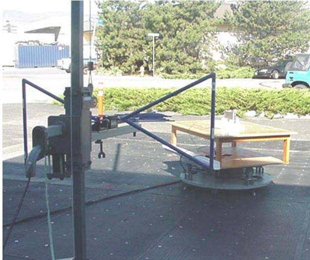
Photograph B.7-1 - Bilog Receive Antenna with DUT Antenna - DUT "Landscape" Configuration
