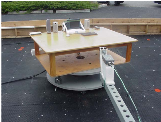
Photograph D-3 - Waveline Horn with LNA @ 1m
