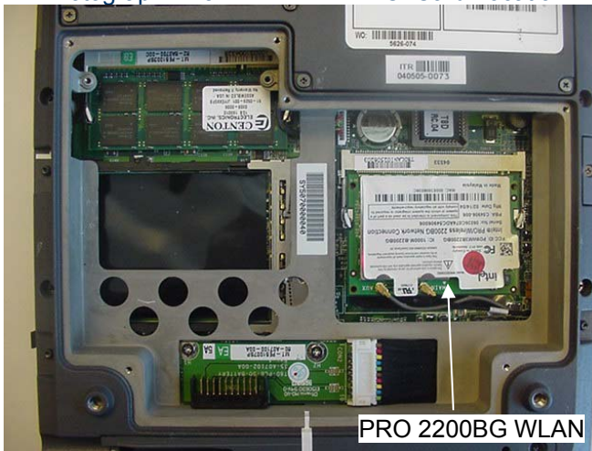
Photograph A-5 - WLAN Mini-PCI Card Location
