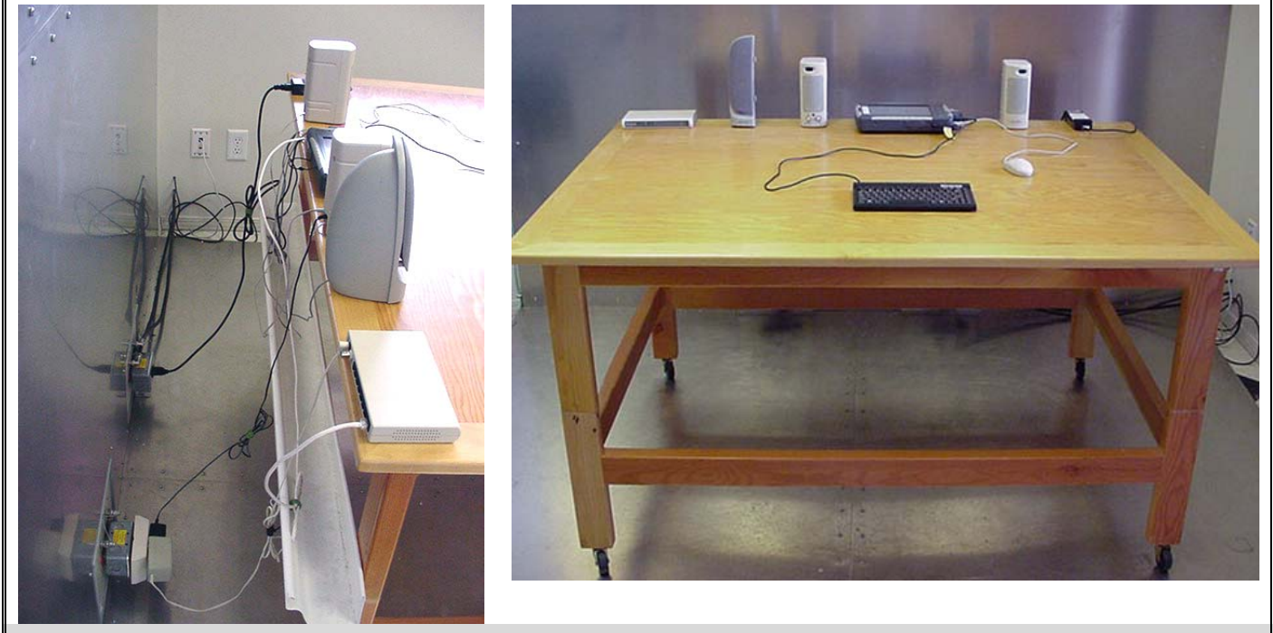
Photograph G-1 - AC Powerline Conducted Emission Cable Placement
