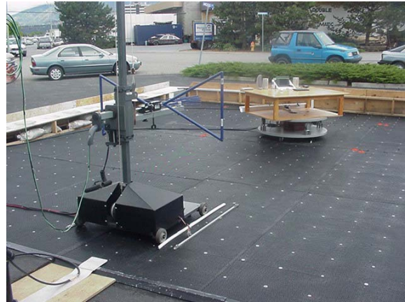
Photograph E-4 - 3115 Horn with LNA/Filter @ 1m
