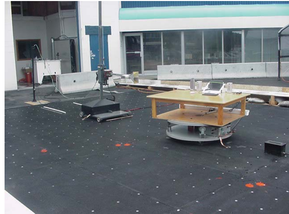
Photograph D-2 - 3115 Horn with LNA/Filter @ 1m
