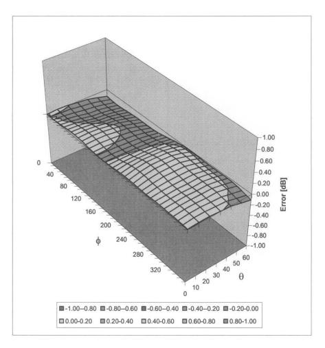
Spherical Isotropy Error < ± 0.4 dB
