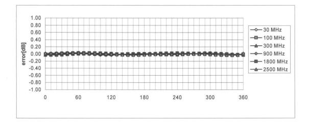
Axial Isotropy Error < ± 0.2 dB
