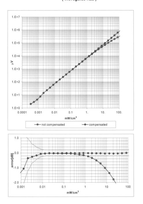
Dynamic Range f(SAR<sub>head</sub>) (Waveguide R22)
