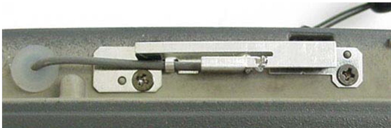
Internal WLAN Antenna 1 (Receive Only)
