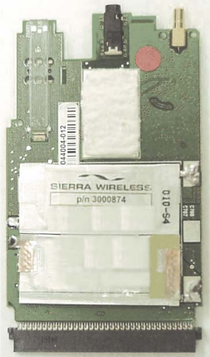
AirCard 775 Dual-Band GSM GPRS/EDGE Modem
