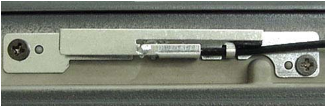
Internal WLAN Antenna 2 (Transmit / Receive)
