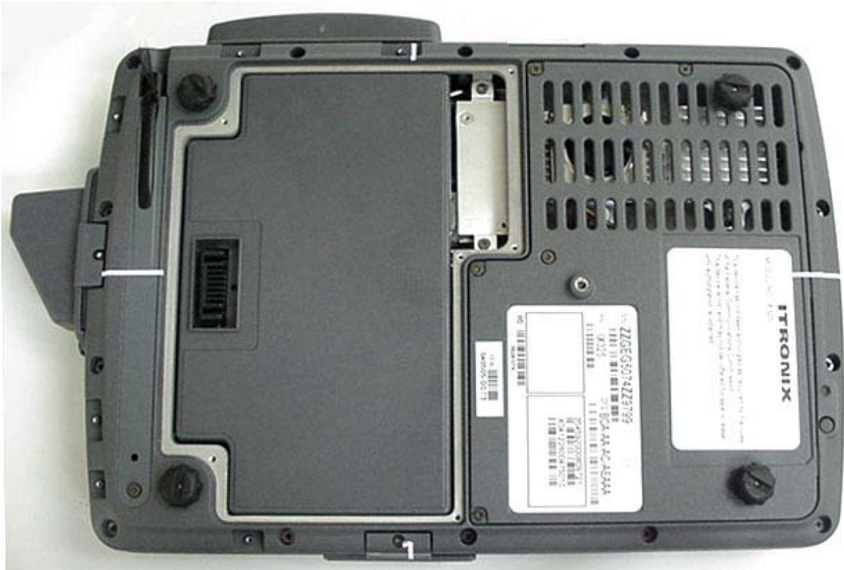
DUT with Internal Li-ion Battery 11.1 V, 3600 mAh (Model: T8M-E)
