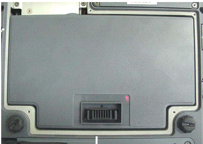
Internal Li-ion Battery 11.1 V, 3600 mAh (Model: T8M-E)
