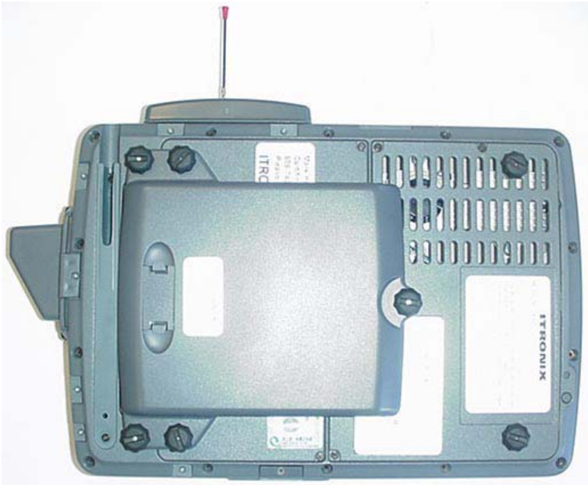
DUT with External Second Li-ion Battery 11.1 V, 3600 mAh (Model: T8S-E)
