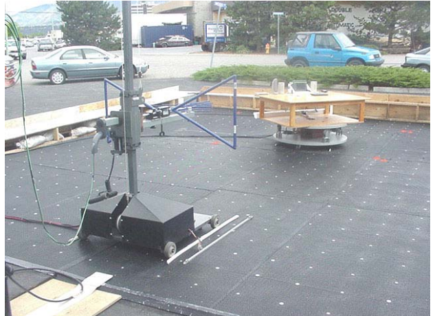
Photograph I.8-4 - 3115 Horn Antenna (2GHz - 10GHz)
