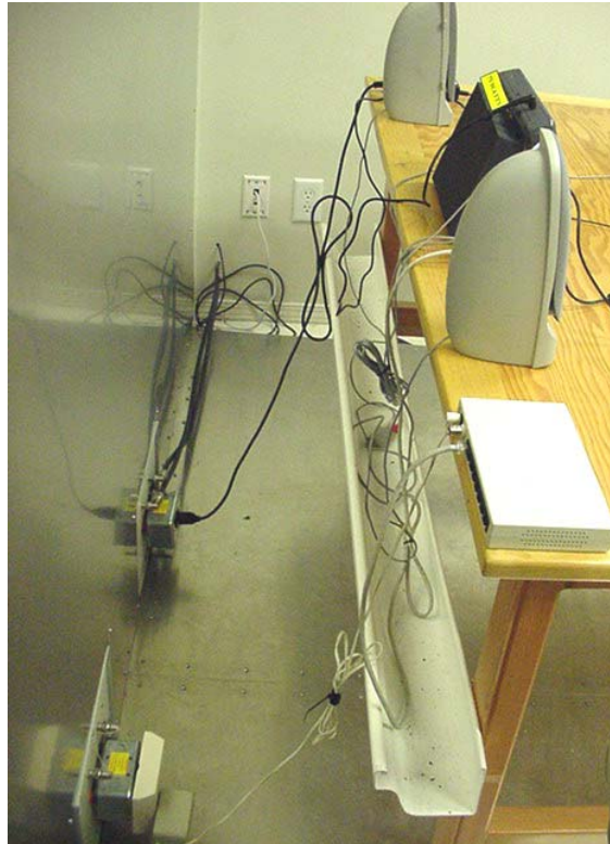
Photograph B.6-2 - AC Powerline Conducted Emission Cable Placement
