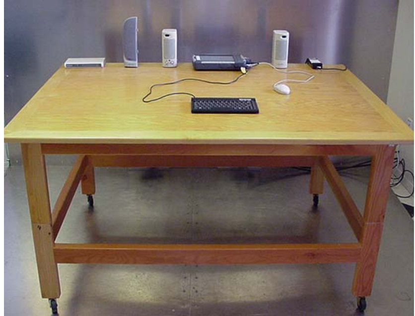
Photograph H-2 - AC Powerline Conducted Emission Configuration
