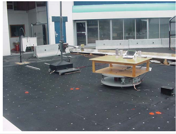
Photograph G-4 - 3115 Horn with LNA/Filter @ 1m
