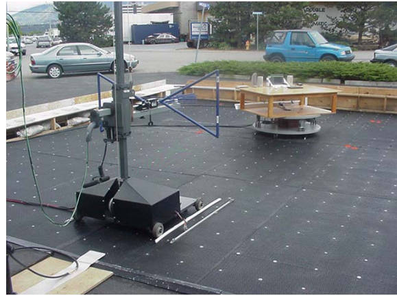
Photograph G-4 - 3115 Horn with LNA/Filter @ 1m
