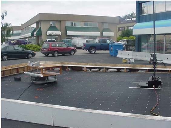
Photograph F-1 - 3115 Horn with LNA/filter @ 3 m
