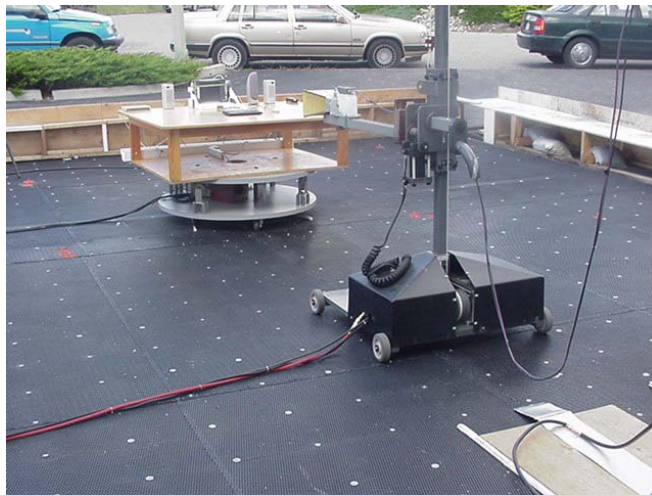
Photograph K.7-3 - Vertical 3115 Horn and LNA PCS Band Radiated Emissions 1-meter Setup
