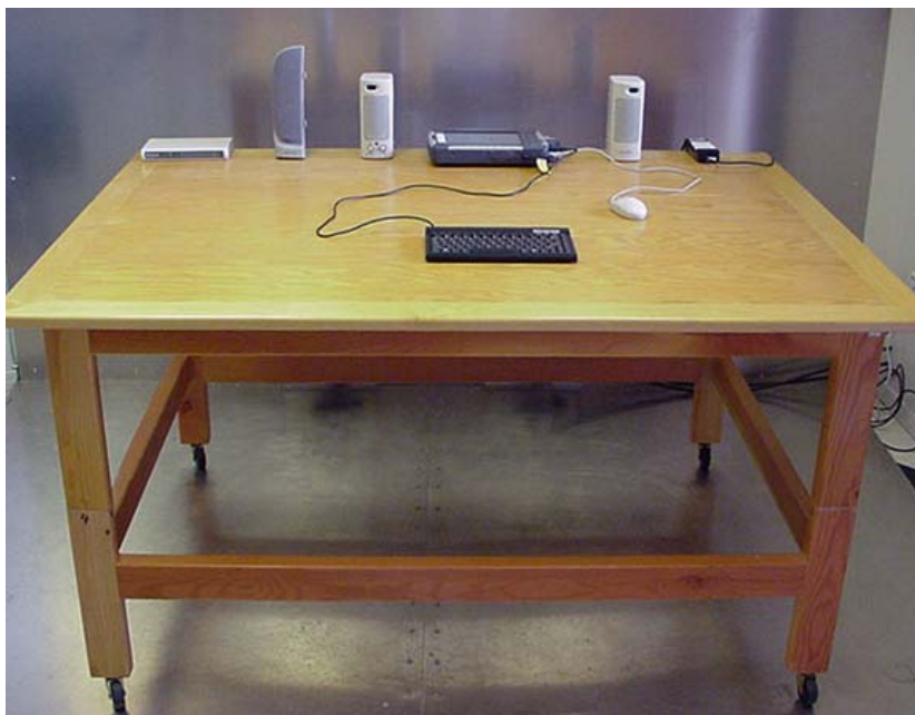
Photograph G-2 - AC Powerline Conducted Emission Configuration
