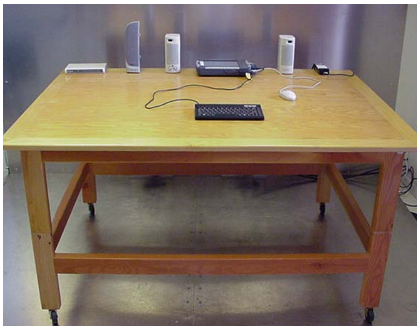
Photograph H-2 - AC Powerline Conducted Emission Configuration
