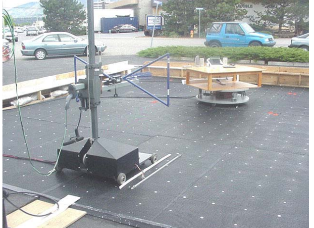
Photograph I.8-4 - 3115 Horn Antenna (2 GHz - 10GHz)
