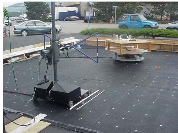
Photograph F-4 - 3115 Horn with LNA/Filter @ 1m
