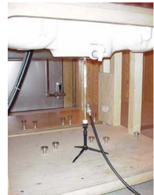
2450MHz Dipole Setup (SAM Phantom)
