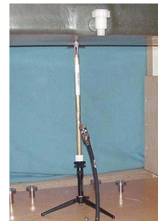
2450MHz Dipole Setup (Planar Phantom)
