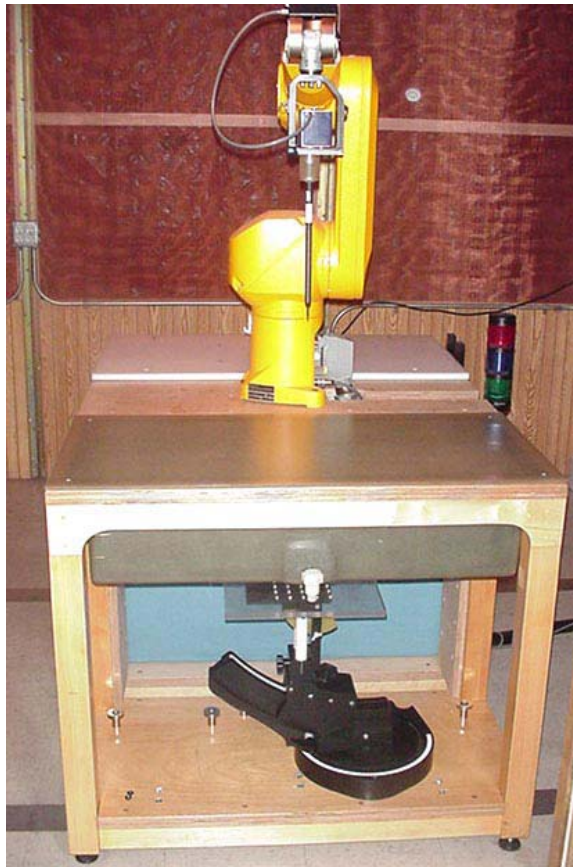
DASY4 SAR Measurement System with planar phantom
