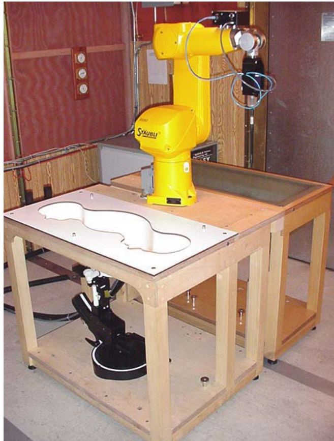
DASY4 SAR Measurement System with SAM phantom
