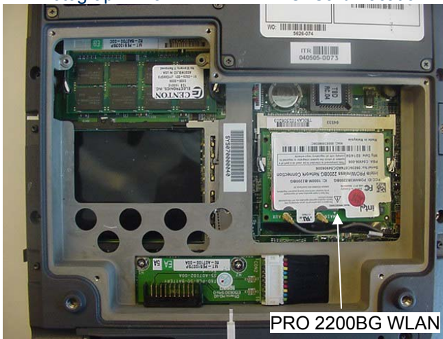
Photograph A-5 - WLAN Mini-PCI Card Location
