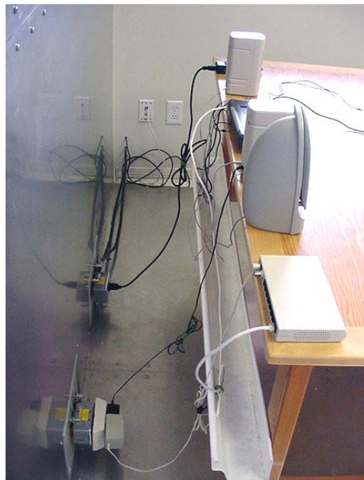
Photograph H-1 - AC Powerline Conducted Emission Cable Placement
