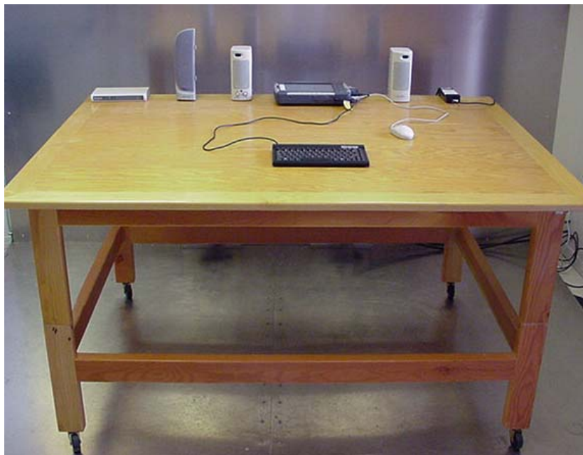
Photograph H-2 - AC Powerline Conducted Emission Configuration
