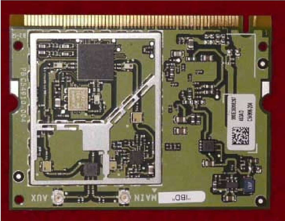
Front with Shielding Removed
