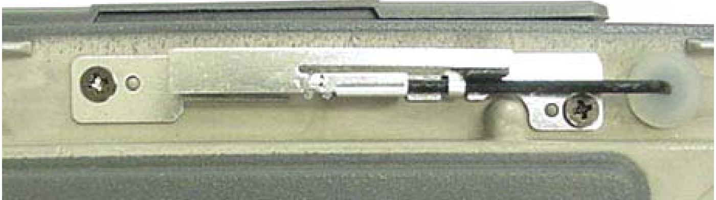
WLAN Antenna 2 (Transmit / Receive)
