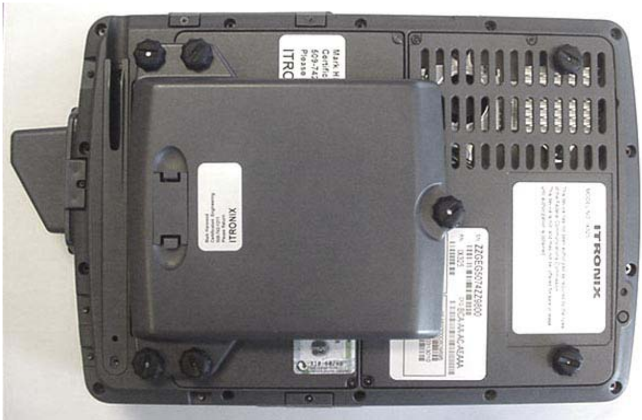
DUT with External Second Li-ion Battery 11.1 V, 3600 mAh (Model: T8S-E)
