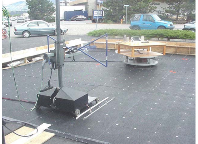
Photograph I.8-4 - 3115 Horn Antenna (2GHz - 10GHz)
