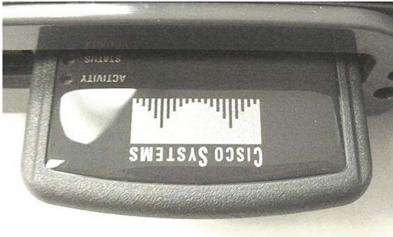
Cisco 802.11abg WLAN Card in PCMCIA Slot (Hatch Cover Removed)
