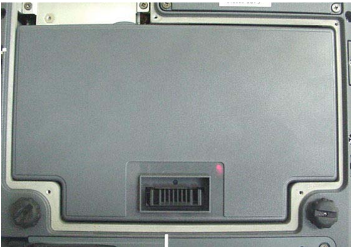
Internal Li-ion Battery 11.1 V, 3600 mAh (Model: T8M-E)
