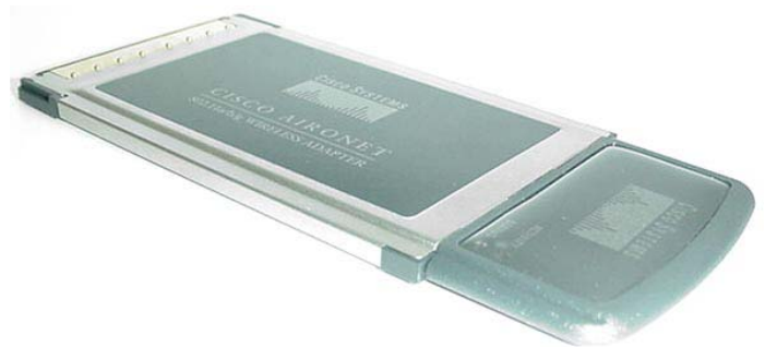
Photograph A-4 - WLAN PCMCIA Card
