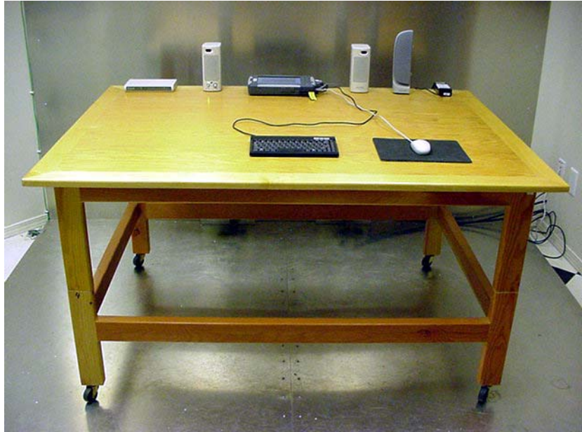
Photograph J-2 - AC Powerline Conducted Emission Configuration
