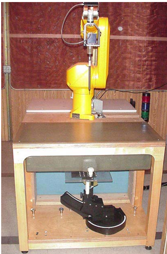
DASY4 SAR Measurement System with planar phantom
