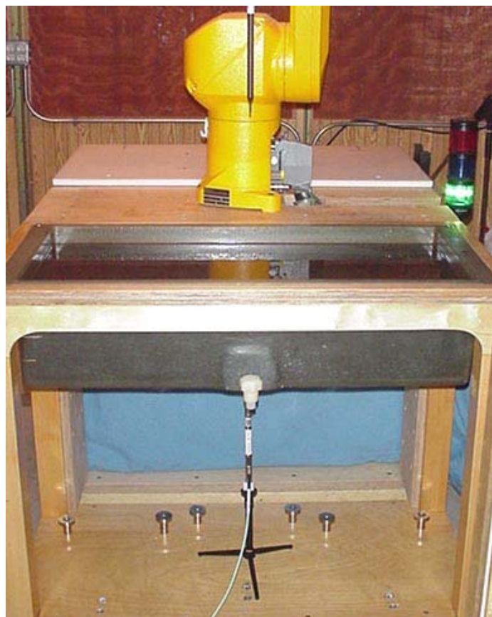
DASY4 SAR Measurement System with planar phantom
