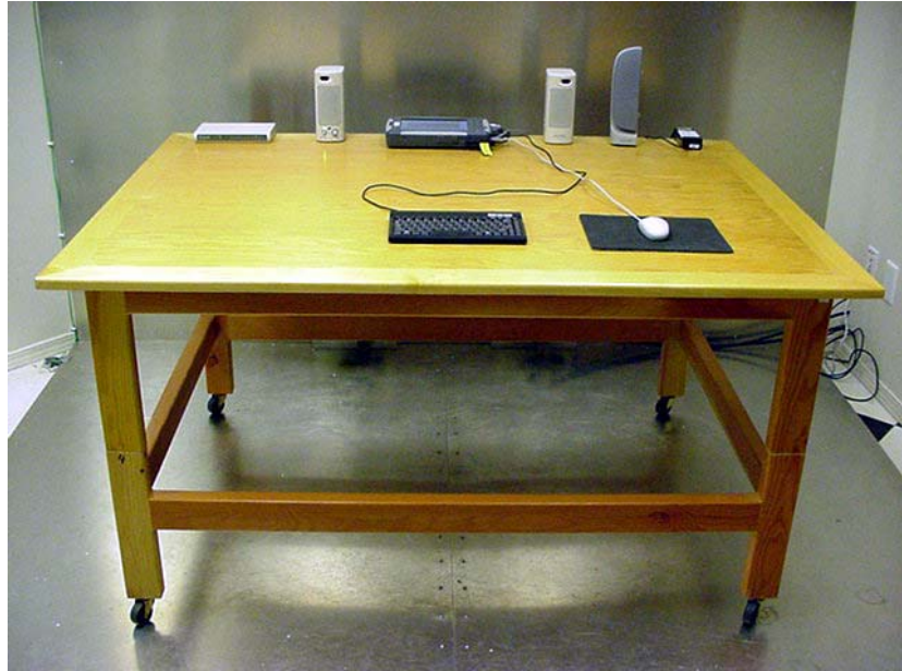
Photograph J-2 - AC Powerline Conducted Emission Configuration
