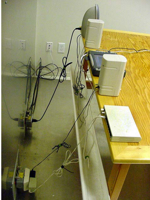
Photograph J-1 - AC Powerline Conducted Emission Cable Placement
