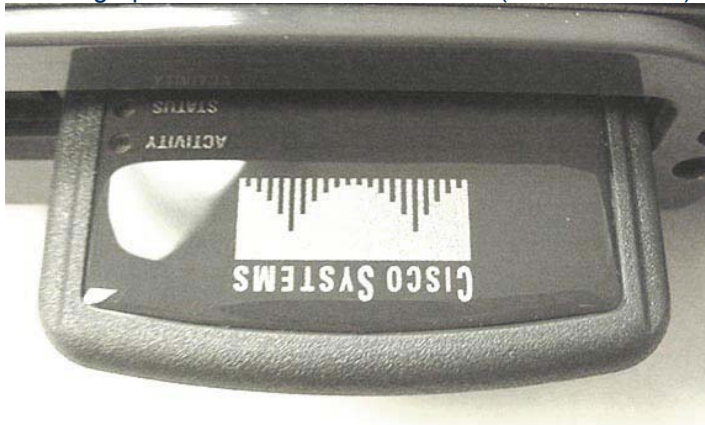
Photograph A-3 - WLAN Card Installed (cover removed)
