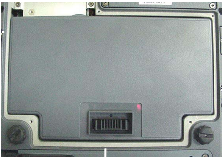
Internal Li-ion Battery 11.1 V, 3600 mAh (Model: T8M-E)
