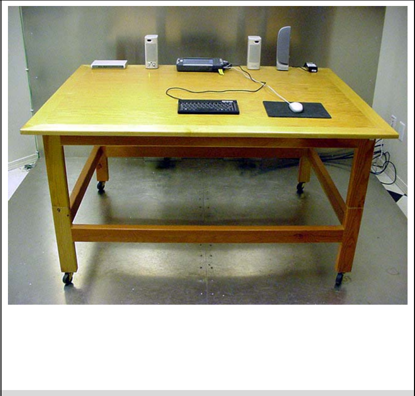
Photograph I-2 - AC Powerline Conducted Emission Configuration
