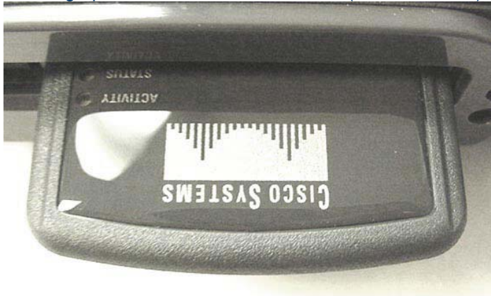
Photograph A-3 - WLAN Card Installed (cover removed)
