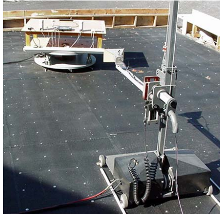
Photograph G-5 - Waveline Horn with LNA @ 1m
