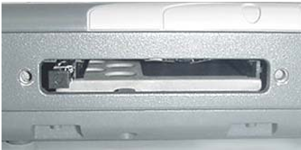
PCMCIA Slot (Low-Profile Hatch & AirCard 860 PCMCIA Card Removed)
