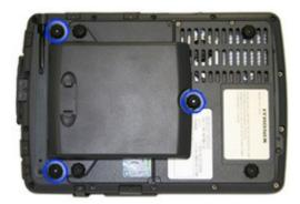
5. Screw the feet into the battery for safekeeping.
