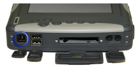
The fax/modem RJ-11 jack can transmit data using the 56 Kbps V.90 or V.92 protocol, and send and receive faxes at 14.4 Kbps. In some countries, local regulations may not permit the use of the fax/modem designed for this system. In this case, you may use a PCMCIA modem.
