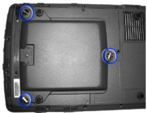
5. Using a Phillips screwdriver, remove the six screws from the battery cover and remove the battery cover.
