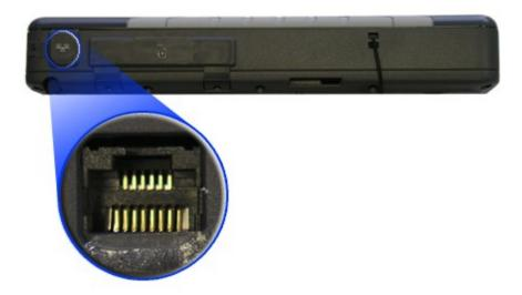
The Ethernet LAN (RJ-45 Jack) on the top edge of the computer enables you to make LAN connections without installing PC cards. Connection speed is 10/100/1000 Mbps.
