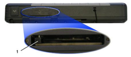
The Duo-Touch has a Type II PC Card Slot located on the top side of the computer. It supports 32 bit Card Bus 2.1 interface as well as Zoom Video when in landscape orientation. You can use this slot to interface between your Duo-Touch and a variety of communications devices, such as network adapters, SCSI adapters, fax/modems, and PC Card Radios. It can also provide additional data storage capacity.
