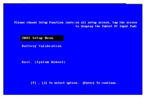
Use your **Line Up** or **Line Down** hot keys to highlight "CMOS Setup Menu" and press the **Enter** key. The system will start the Setup Utility and display the main menu of the utility.
