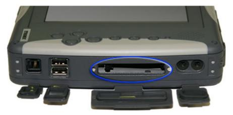
Your Duo-Touch can use Type 1 CompactFlash Cards for secure data storage. If you store any user-installed application programs and associated data on CompactFlash, these programs and data will not be lost after a hard reset. Files stored on CompactFlash Cards can be created, deleted, moved and amended in exactly the same manner as files stored in memory.
