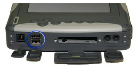
The two Universal Serial Bus (USB) 2.0 ports enable you to attach USB devices such as keyboards, mice, scanners, and printers. USB devices can be chained together on a single cable.
