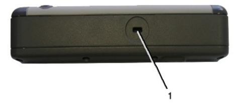
Your computer has a Security Slot (1) on the left side. It can be used with a standard laptop locking device, such as a Kensington Lock. You can connect the Duo-Touch to a large object with the lock to prevent theft of your Tablet PC. See the documentation that comes with your lock for more information.
