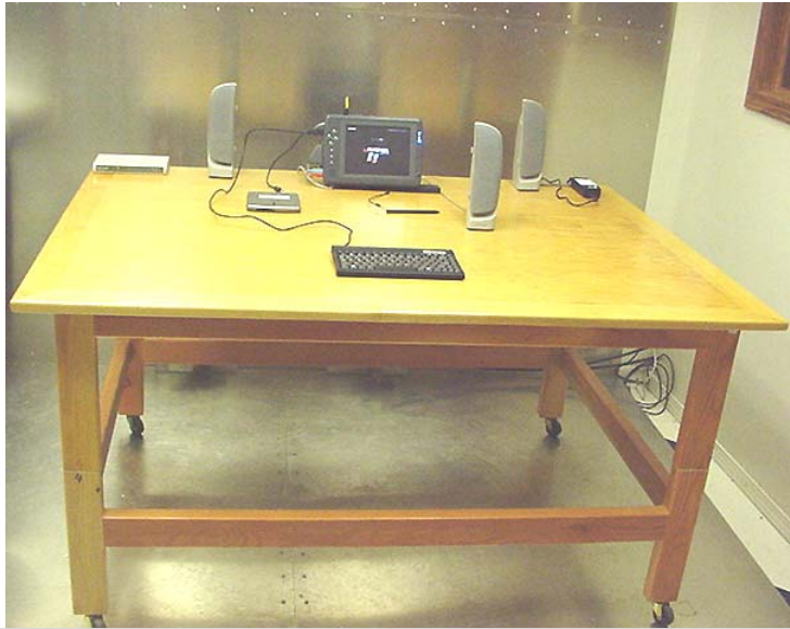
Photograph B.6-2 - AC Powerline Conducted Emission Cable Placement
