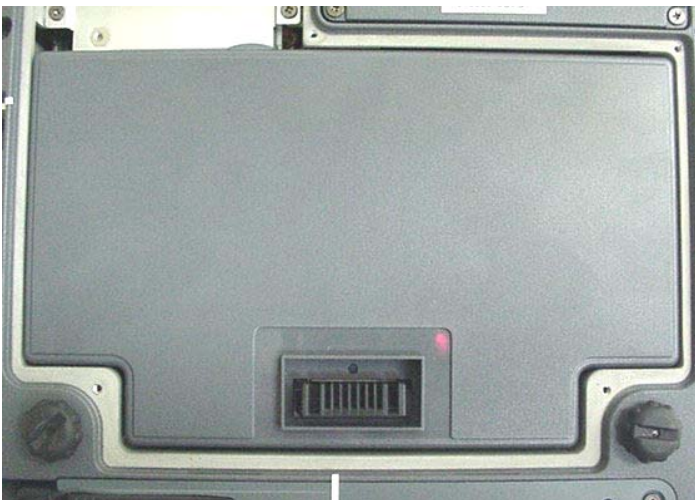
Internal Li-ion Battery 11.1 V, 3600 mAh (Model: T8M-E)
