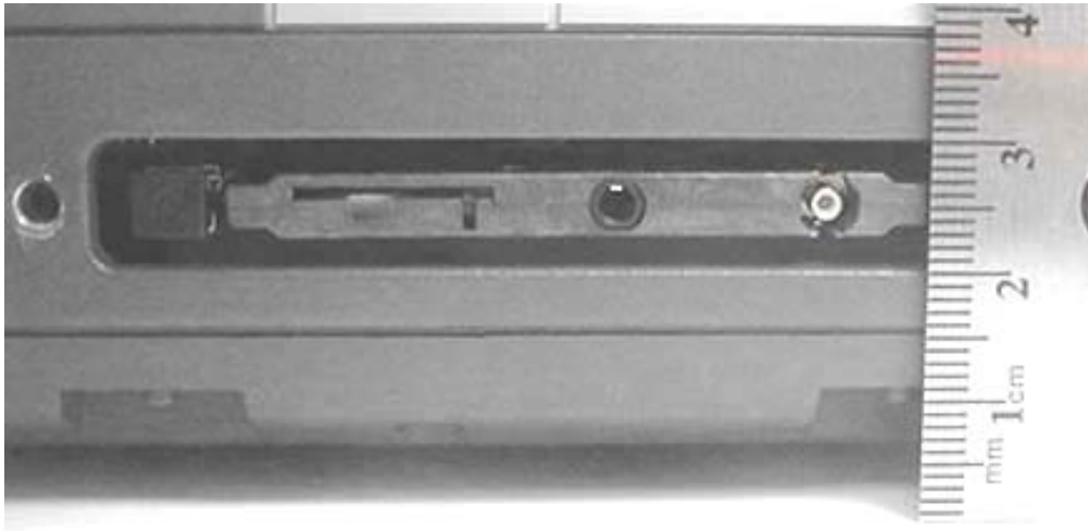
PCMCIA Slot-to-Base Distance (Low-Profile Hatch & AirCard 860 Antenna Removed)
