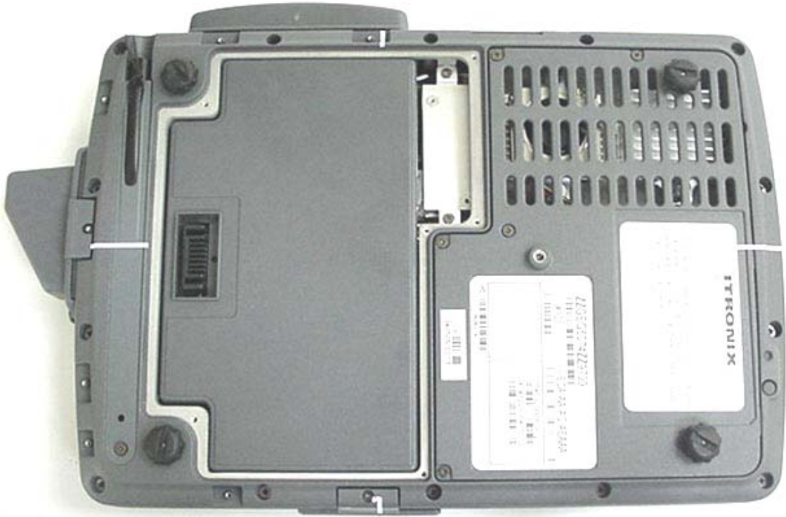
Bottom Side of DUT with Internal Li-ion Battery 11.1 V, 3600 mAh (Model: T8M-E)
