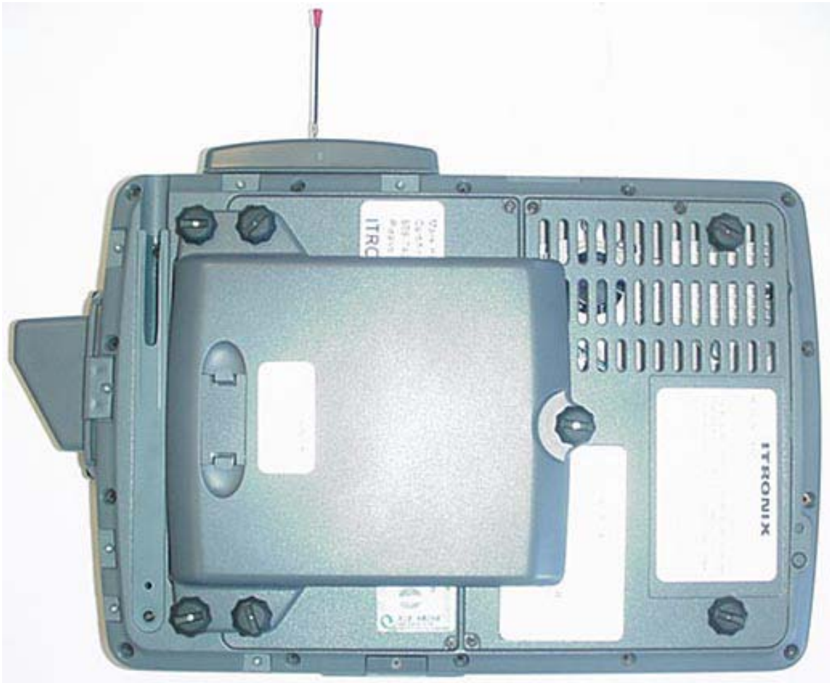
Bottom Side of DUT with External Second Li-ion Battery 11.1 V, 3600 mAh (Model: T8S-E)
