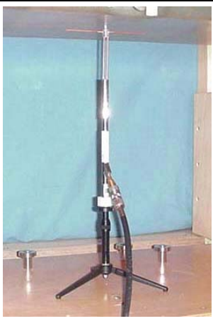
835MHz Dipole Setup
