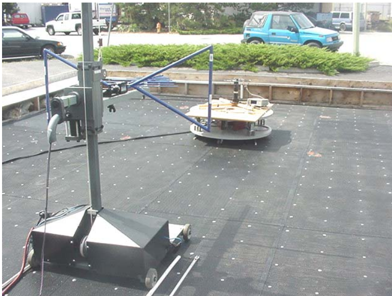
Photograph B.7-3 - Dipole Substitution Setup
