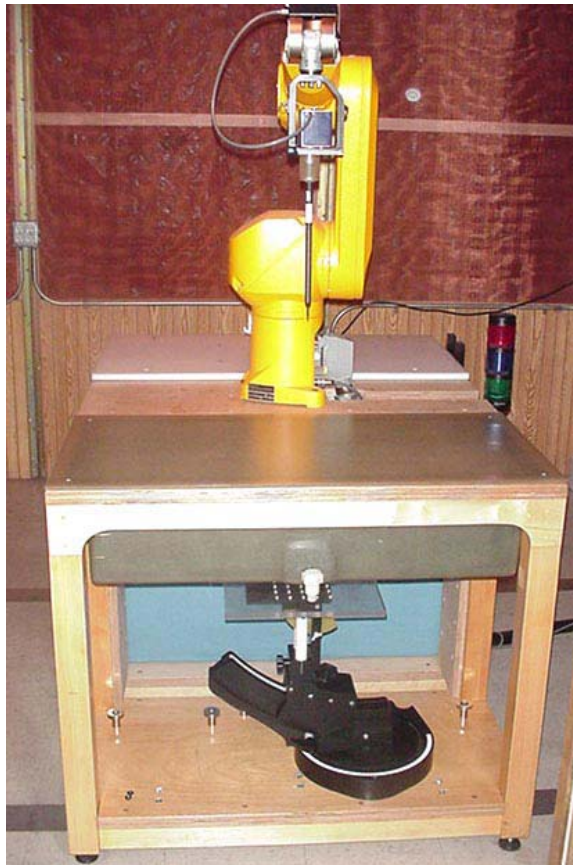
DASY4 SAR Measurement System with planar phantom
