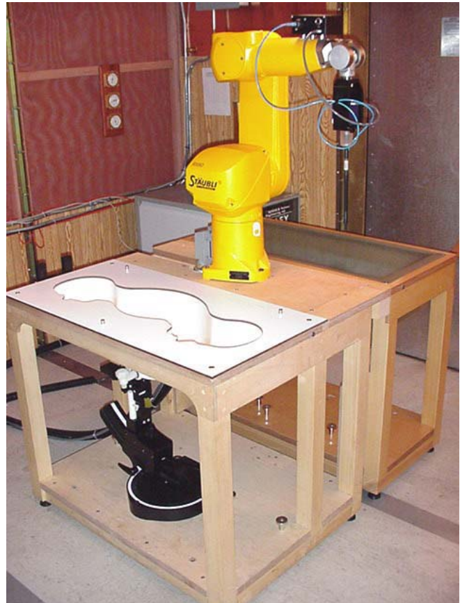
DASY4 SAR Measurement System with SAM phantom
