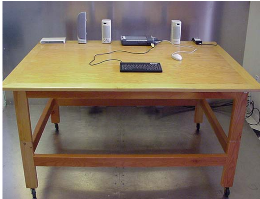
Photograph G-2 - AC Powerline Conducted Emission Configuration
