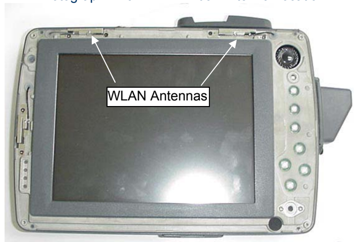
Photograph A-6 - WLAN Dual Antenna Location
