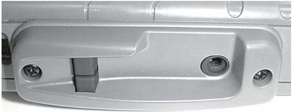
IX325 Hatch for AirCard 775 (Antenna Removed)
