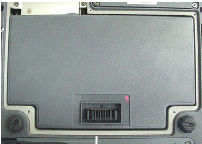
Internal Li-ion Battery 11.1 V, 3600 mAh (Model: T8M-E)
