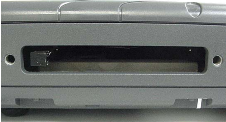
PCMCIA Slot (Hatch & AirCard 775 Removed)
