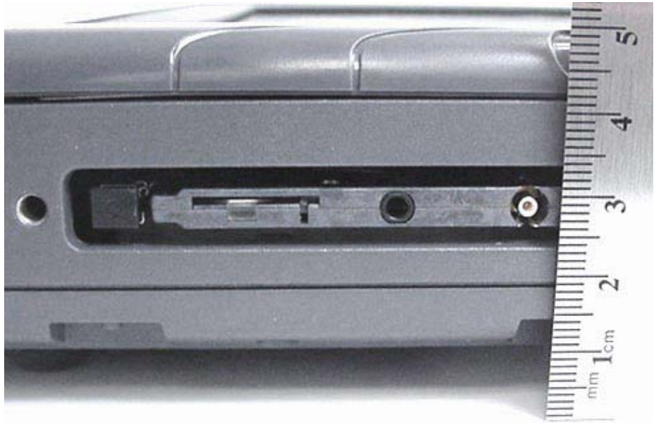
PCMCIA Slot-to-Base Distance (Hatch & Antenna Removed)
