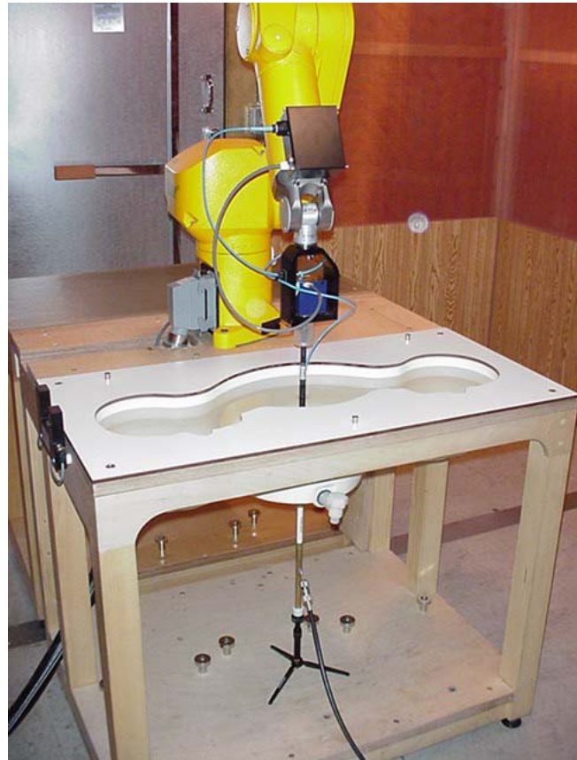
DASY4 SAR Measurement System with SAM phantom
