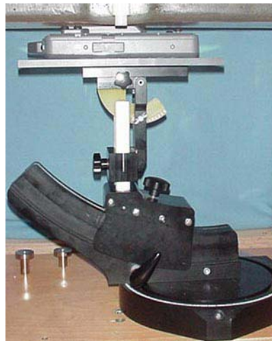
DUT Test Setup with External 2 nd Battery
